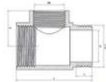
BATARYA UZATMASI (DELİKLİ) FAUCET EXTENSION (HOLE)
